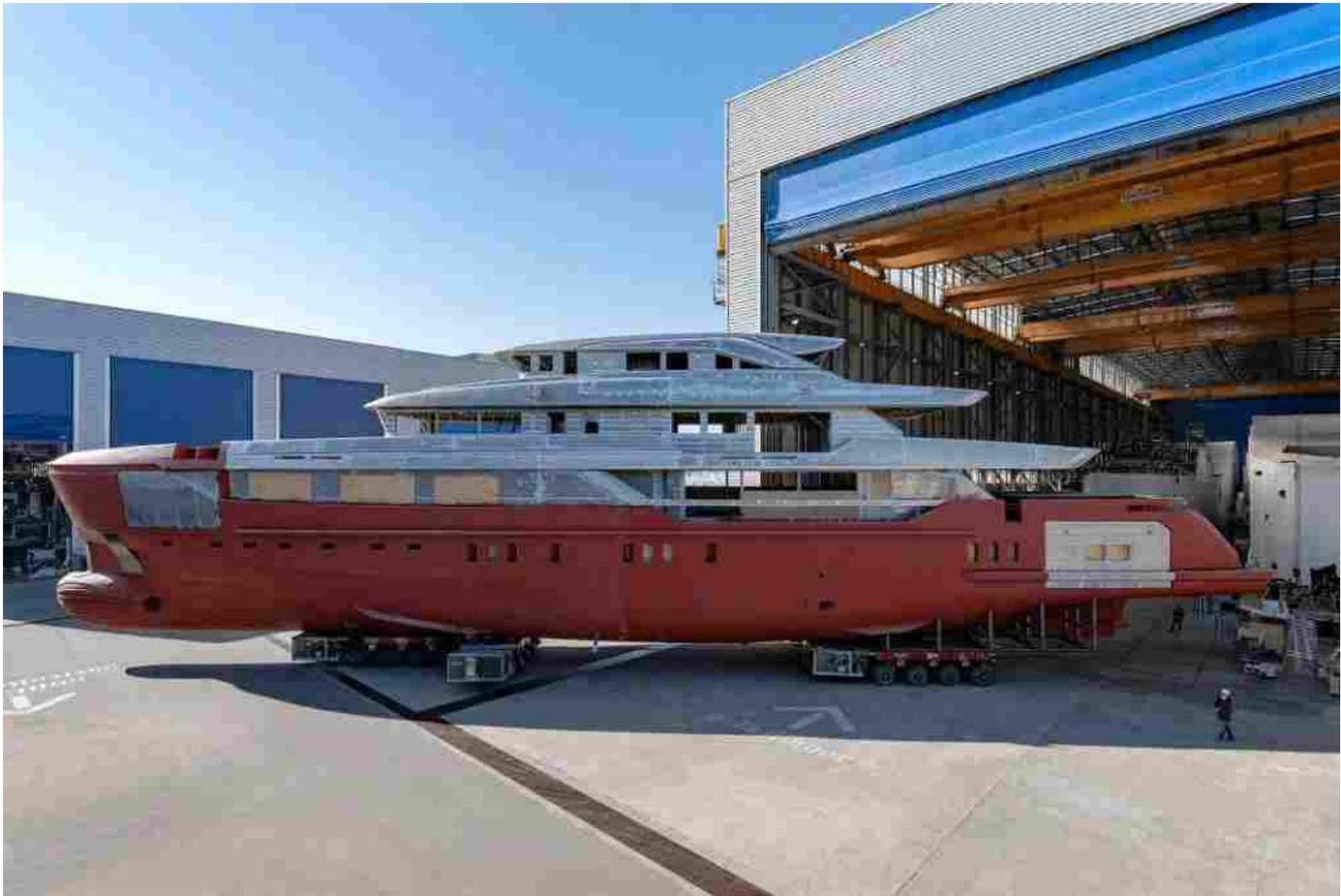
*The 57Steel has five levels including a full bridge deck*
