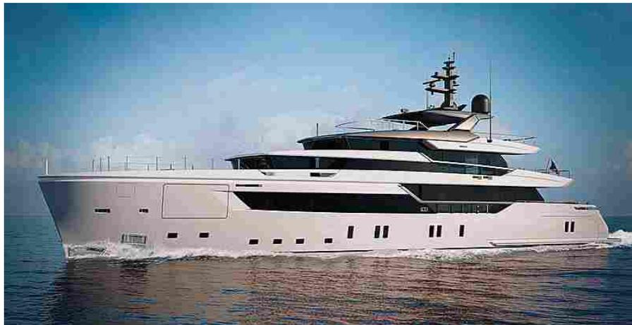
The 44.5-metre Alloy motor yacht is constructed entirely of aluminium and is the result of a collaboration between Bernardo Zucon of [Zucon International Project](#) and Sanlorenzo's in-house design team. The motor yacht sits just below the 500 GT mark at 485 GT and is spread across three decks with ample space both externally and internally.
