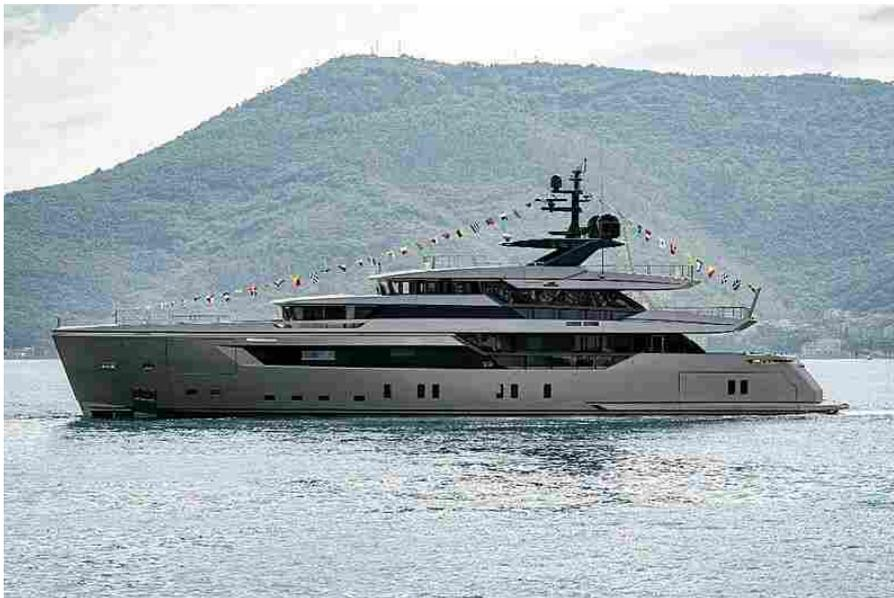
The unparalleled privacy of the owner's suite has been achieved with the use of a 'ziggurat' deck layout, which means that it is not possible to overlook the owner's deck, even from the wheelhouse above.
