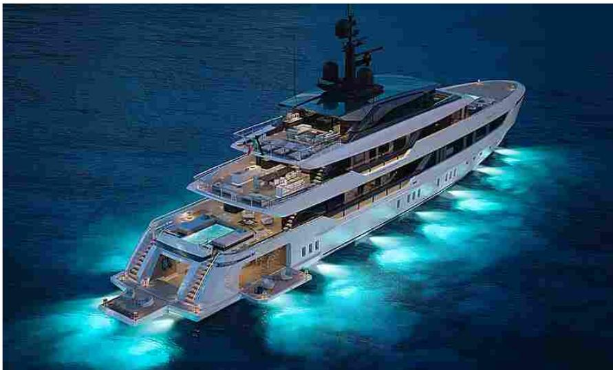
The 57Steel can be equipped with a hybrid diesel-electric propulsion system. With her standard [Caterpillar 3512C](#) diesel engines, she can reach a top speed of 16.5 knots and a cruising speed of 12.5 knots. She has a range of 4,000 nautical miles while cruising at 11 knots.
